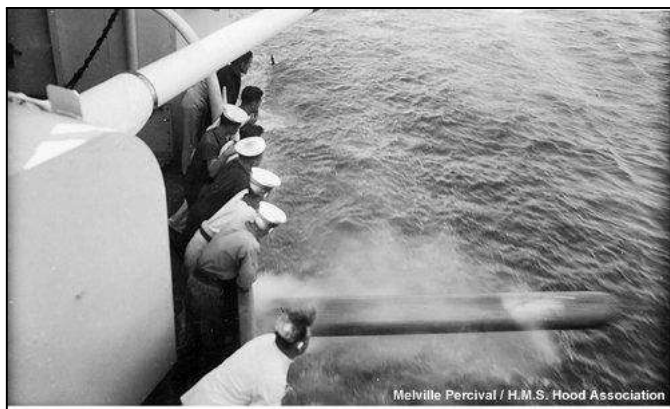
A 21-inch torpedo fired from one of the above water tubes (Percival Collection, H.M.S. Hood Association)
